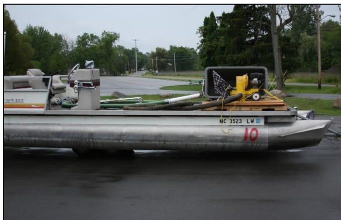
Figure 40. A DASH boat for hand-removal of watermilfoil or other nuisance vegetation. ©Restorative Lake Sciences, LLC
